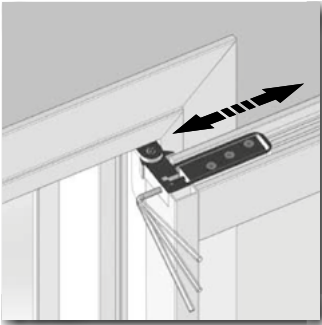
Fast and easy regulation for lateral alignment of the door.
